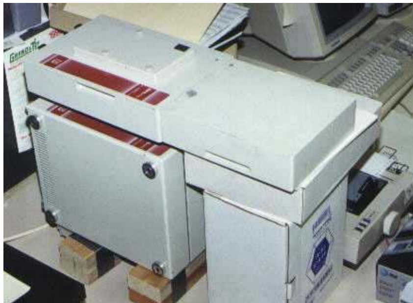
Fig. 1. Foss NIRSystems model 6500 visible/near-infrared scanning spectrophotometer on its back so that the sample transport (uppermost) operated horizontally instead of vertically.
