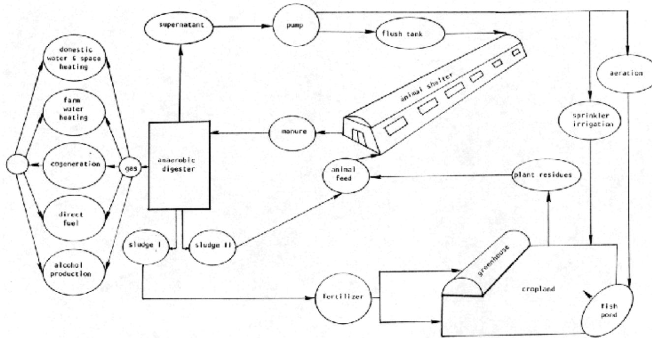
Figure 7. An efficient farm-energy system through biodigestion.
