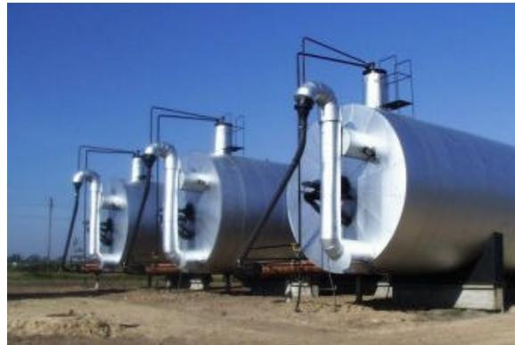
*left picture* Manure inlet, mixer tanks, agitator motors/gears. *right picture* Manure outlet, gas outlet.
