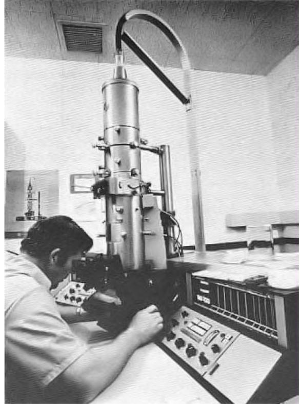
Electron microscope analysis for asbestos fibers at Duluth EPA Laboratory.
