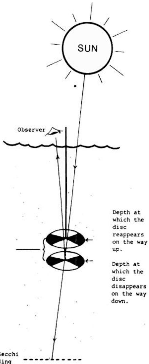
FIGURE 1: Use of Secchi Disc to determine water clarity.
