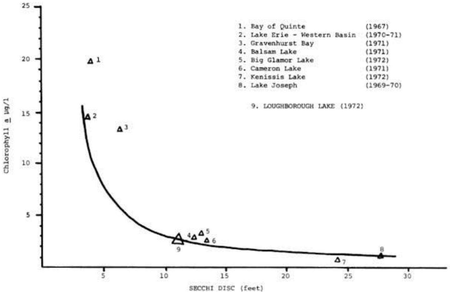
**Figure 6:** The mean of chlorophyll  $a$  and Secchi Disc measurements in Loughborough Lake relative to a curve describing the chlorophyll  $a$  - Secchi disc relationship in many Ontario lakes. Eight other well known lakes are included for comparison with Loughborough Lake.
