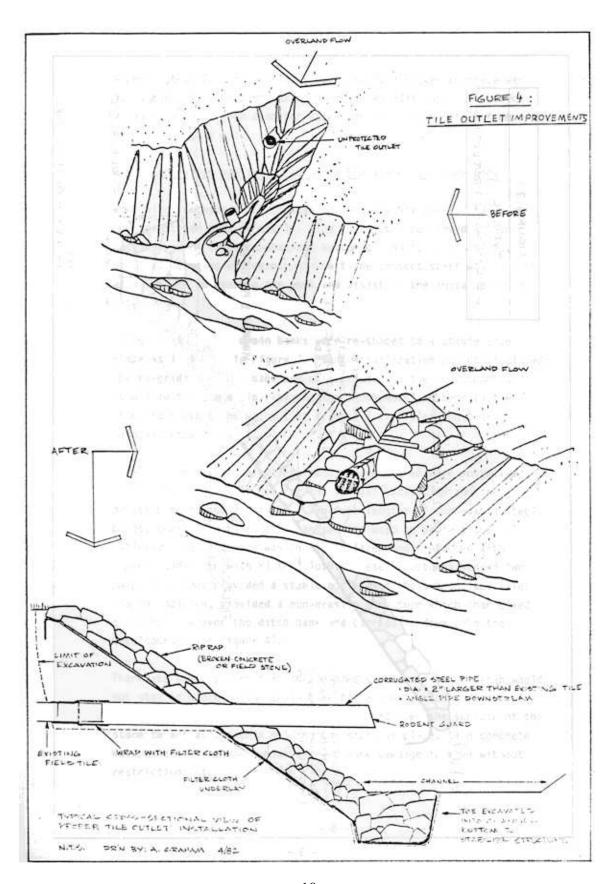
The remaining two tile outlets on Lot 16 were installed manually by project staff. This involved the connection of the steel outlet pipes to the tiles and provision of stone rip-rap around the outlet to secure the pipe and prevent scouring.
