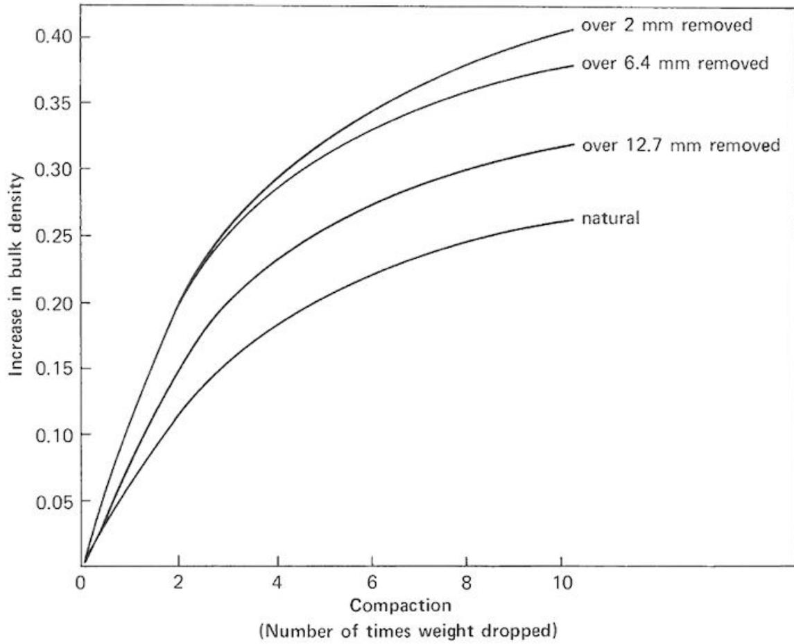
**Fig. 1.** Effect of stones on soil compactibility (Struchtemeyer 1960).
