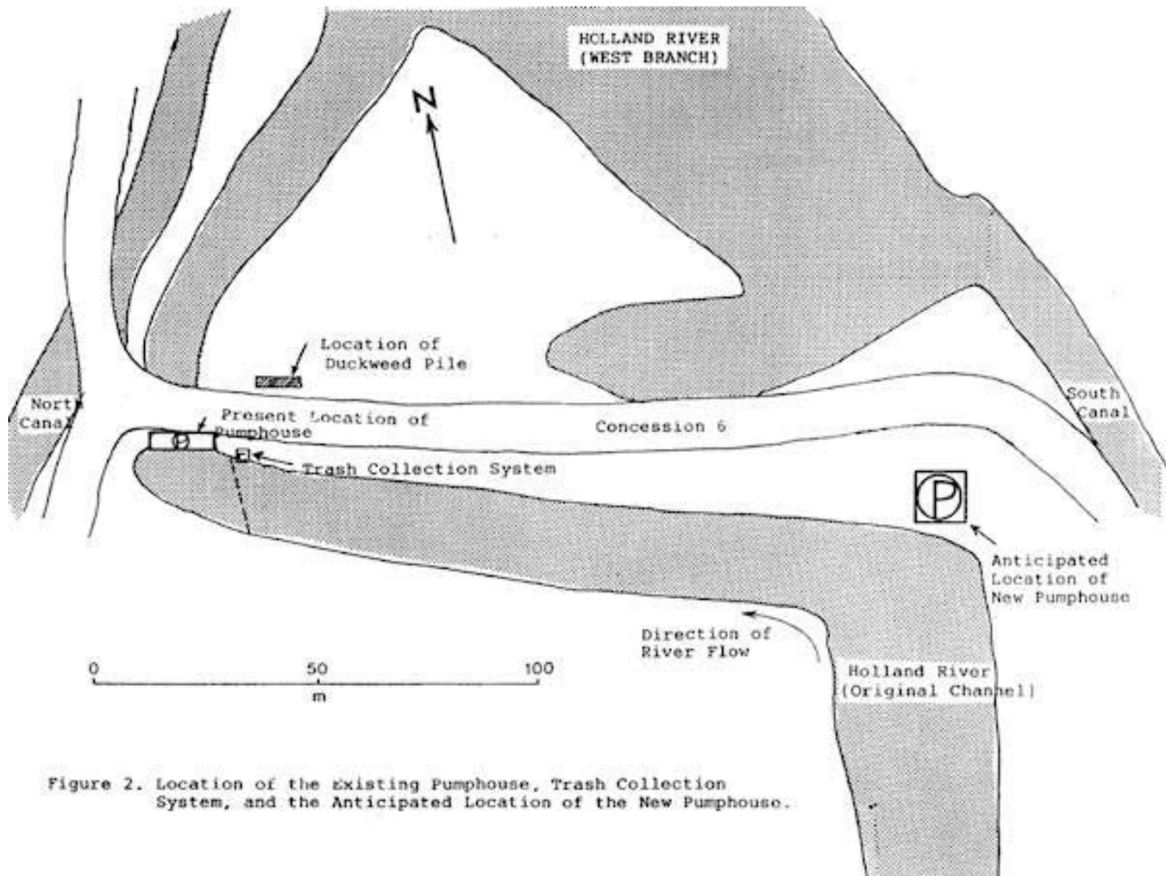
Figure 2. Location of the Existing Pumphouse, Trash Collection System, and the Anticipated Location of the New Pumphouse.
