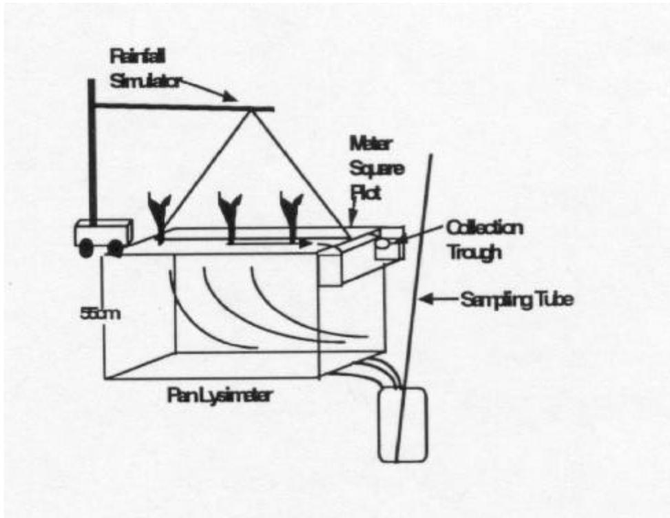
**Figure 1.** Diagrammatic vertical cross section of experimental setup.
