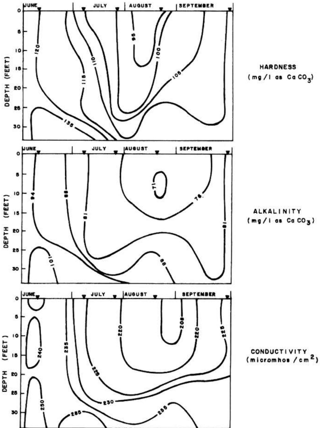
**FIGURE 3:** Isopleths of Hardness Alkalinity and Conductivity at Station "A" Roblin Lake June 9<sup>th</sup> - Sept. 30<sup>th</sup> , 1970.
