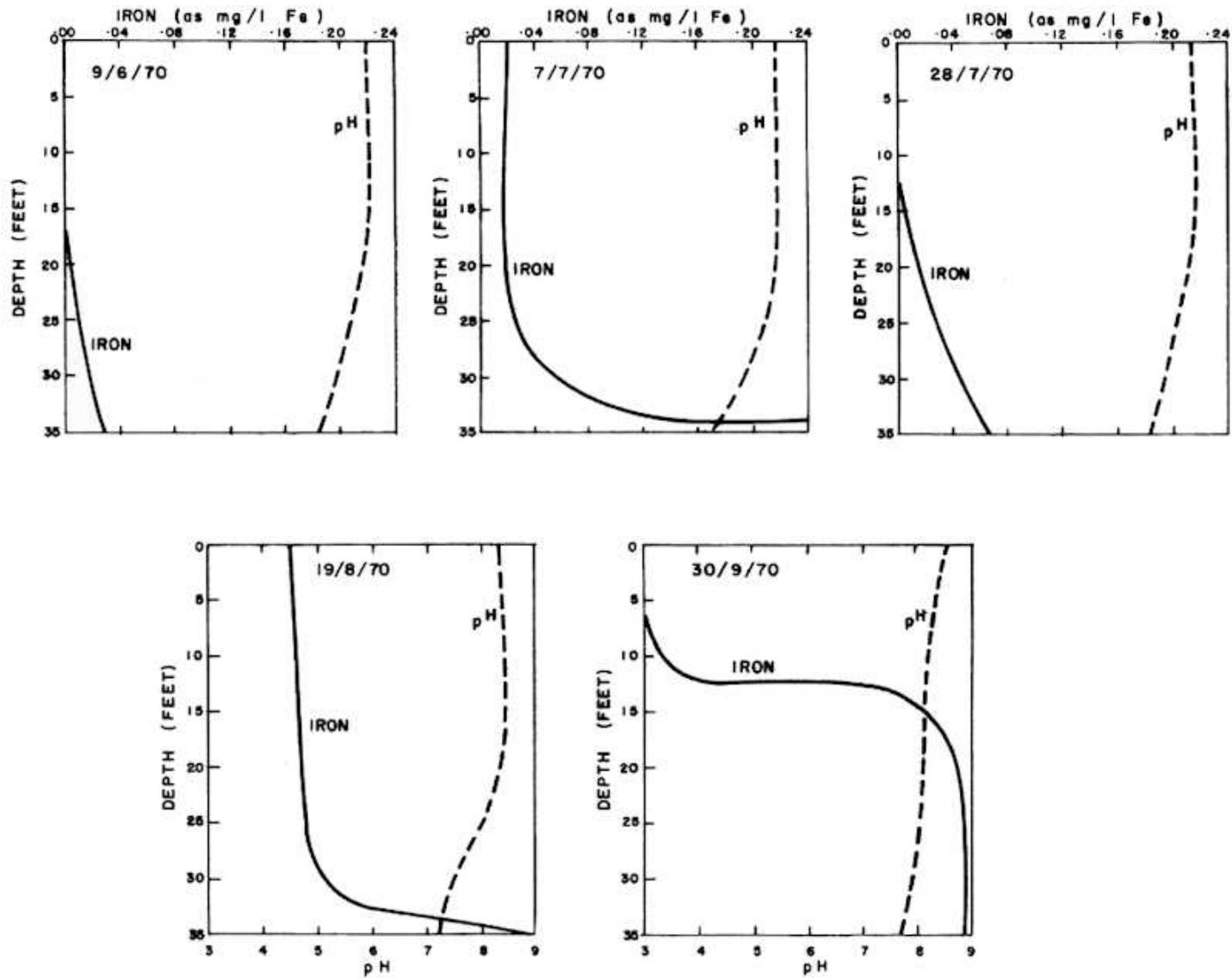
**FIGURE 4:** Profile Of Iron (as mg /L Fe) and pH on five dates in 1970 at Station "A" Roblin Lake.
