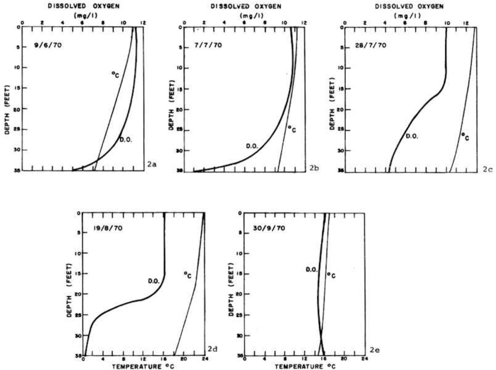
**FIGURE 2:** Profiles of Dissolved Oxygen (Mg/L ) And Temperature °C on Five Dates in 1970 at Station "A" Roblin Lake at the surface and 18.5°C at the bottom; corresponding readings on September 30<sup>th</sup> were 17.5°C and 16.0°C (Figure 2).
