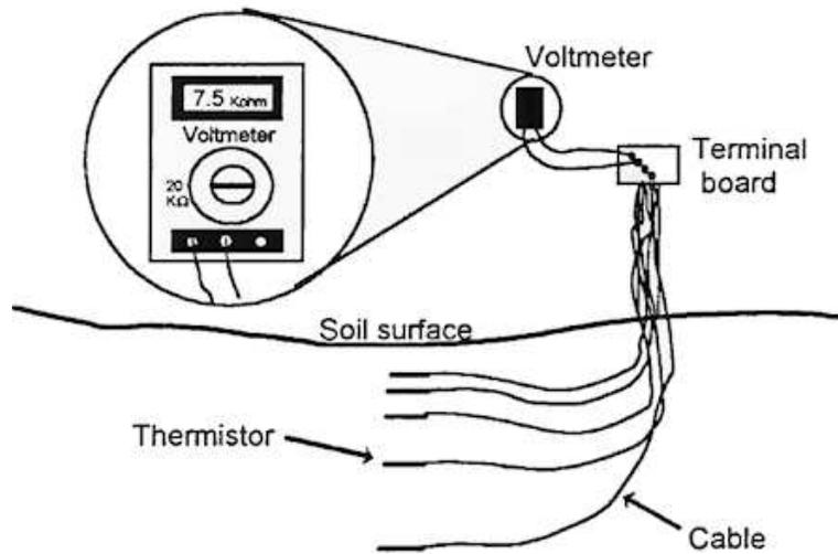
**Figure 20.** Thermistor and voltmeter system.
