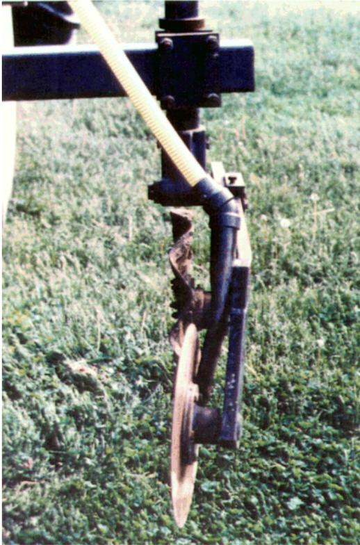
Front view of coulters and disc opener for left side of Row 1
