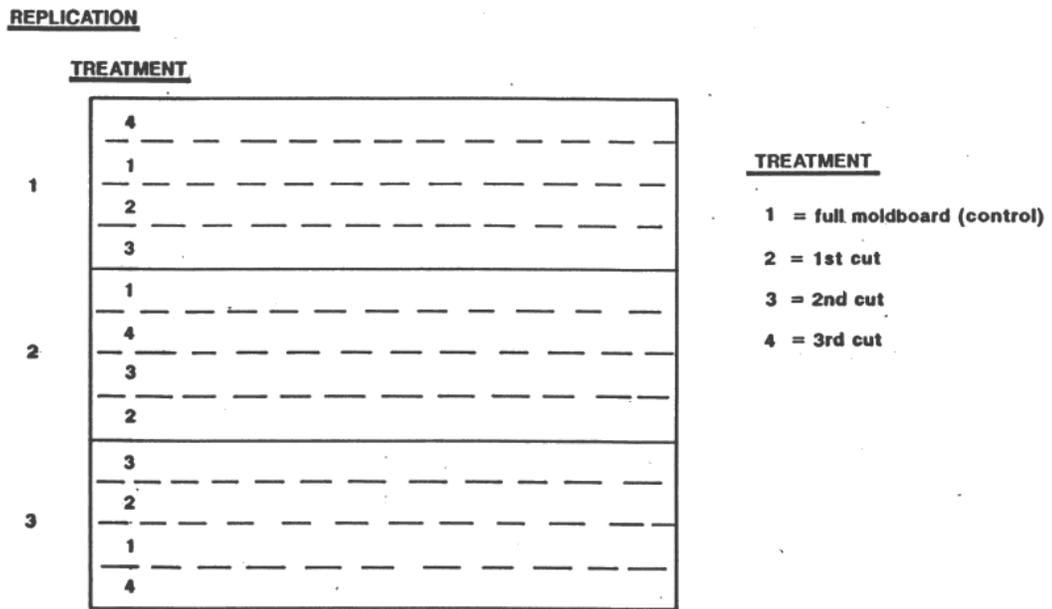
**Figure 2.** BASIC DESIGN of MOLDBOARD MODIFICATIONS used in 1989 TRIALS
