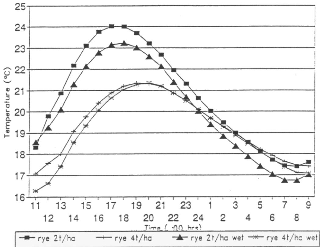
**Figure 2.4** Temperature lows for all rye treatments (June 14-15, 1988)
