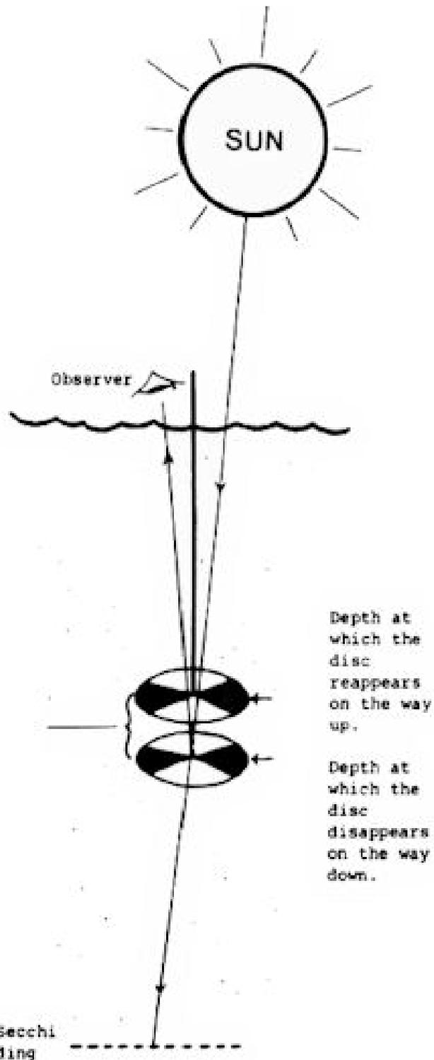
FIGURE 1: Use Of The Secchi Disc To Determine Water Clarity.
