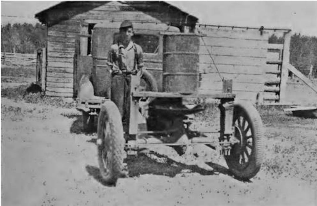
**FIG. 14.** Bait spreader using discarded disk from one-way disk for spreader table.
