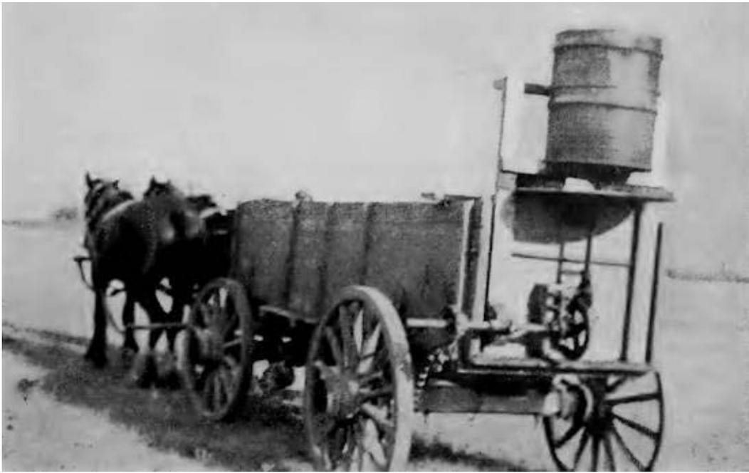
**FIG. 3.** Endgate bait spreader.
