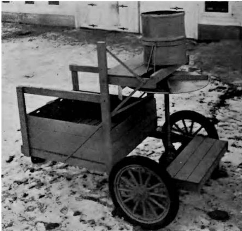
**Fig. 6.** Autotrailer bait spreader.
