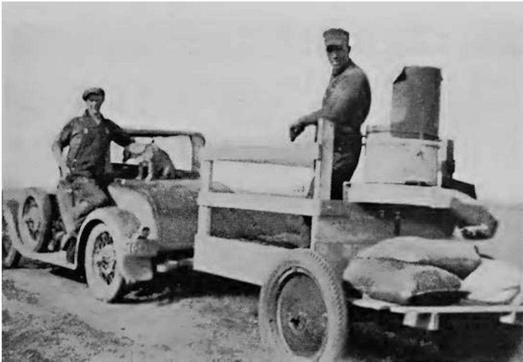
**FIG. 5.** Autotrailer bait spreader.
