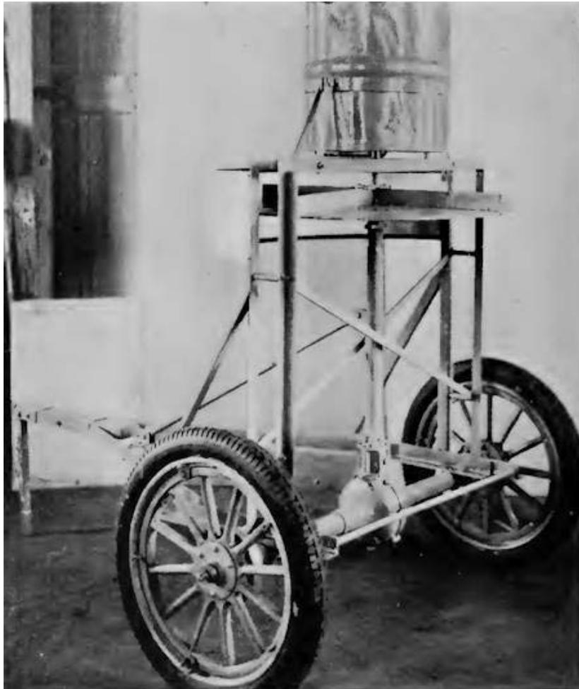
**FIG. 12.** Truck-trailer bait spreader (rear).
