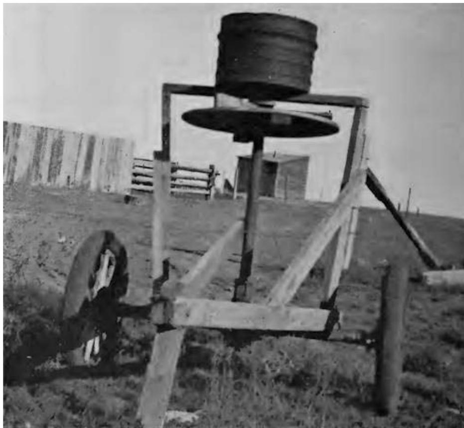
**FIG. 13.** Truck-trailer bait spreader with wood frame.
