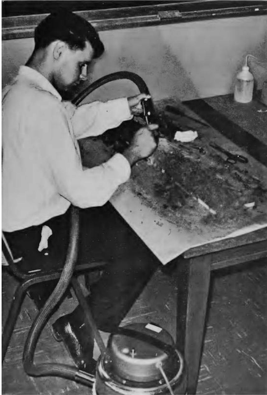
**Fig. 9.** Loosened soil is removed with a vacuum cleaner.
