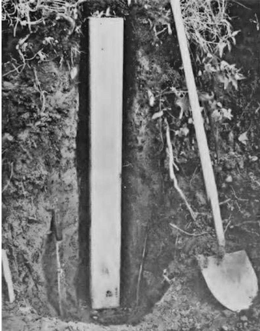
**Fig. 2.** The wooden box is carefully placed over the column of soil.
