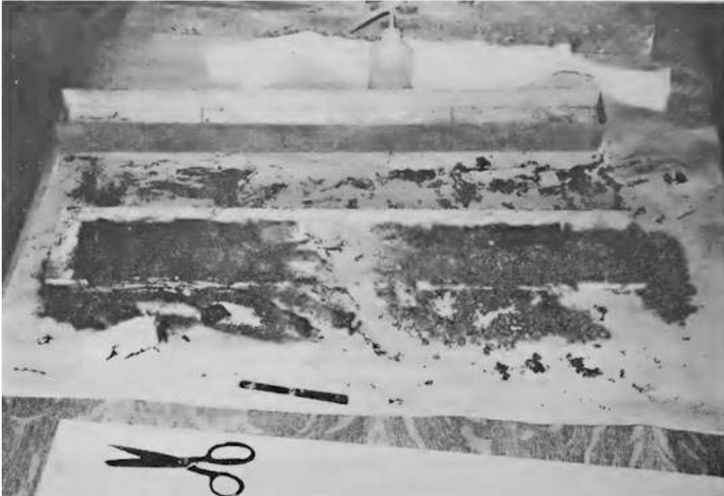
**Fig. 8.** The sheet-metal box has been removed and the monolith is on the resin-coated board.
