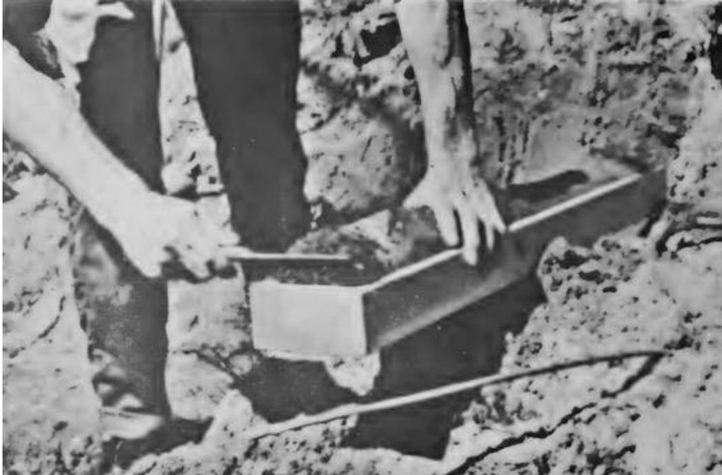
**Fig. 5.** Excess soil is removed from the monolith.
