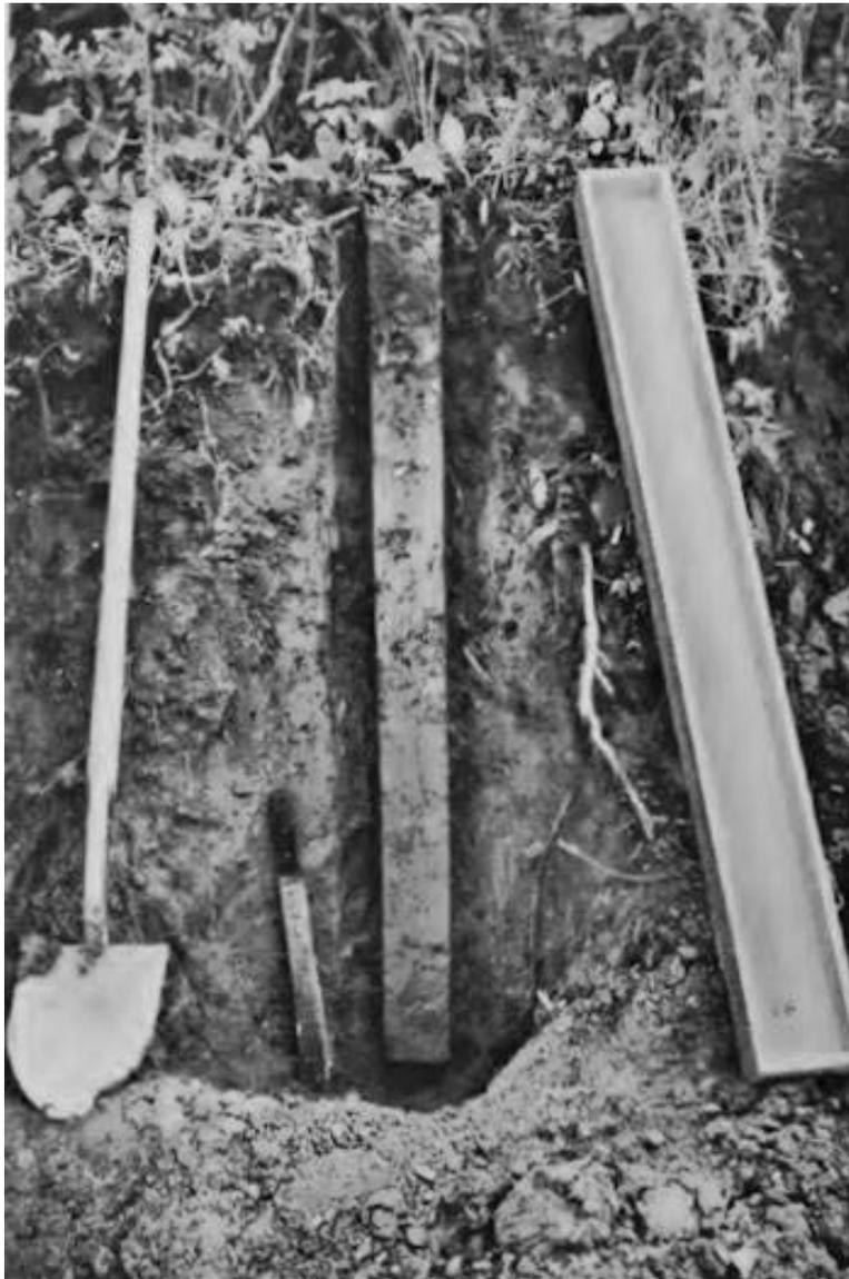
**Fig. 1.** The trimmed column of soil is ready to be fitted into the wooden box.
