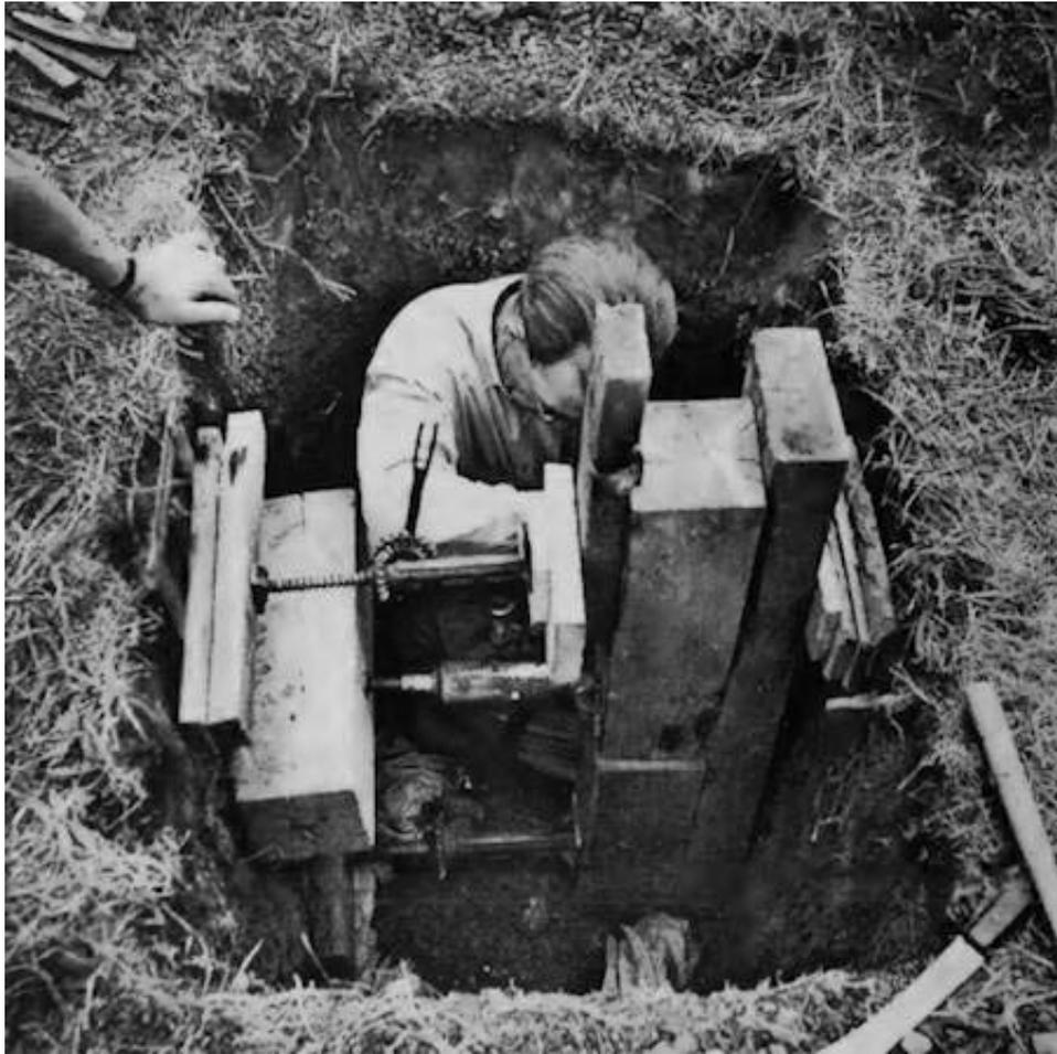
**Fig. 3.** The angle-iron frame without its backing board is forced into the soil by means of three screw jacks.
