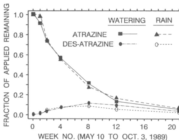
**Fig. 6.** Mobility profiles for atrazine and desethylatrazine (Des-Atraz.) in Plainfield sand lysimeters treated with metribuzin under both supplementary watering and rainfall.
