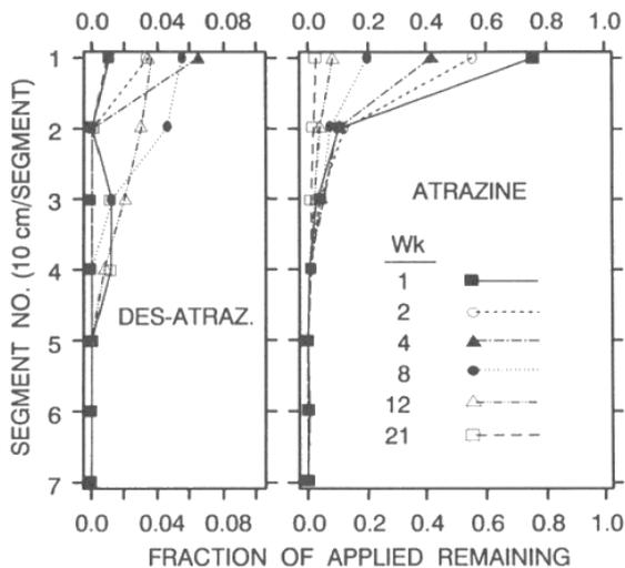
**Fig. 5.** Mobility profiles for atrazine and desethylatrazine (Des-Atraz.) in Plainfield sand lysimeters treated with metribuzin under supplementary watering.
