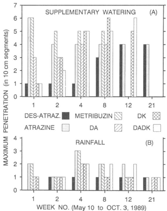
**Fig. 2.** Maximum penetration of atrazine, desethyl-atrazine (Des-Atraz.), metribuzin, DA, DK, and DADK in Plainfield sand lysimeters: (A) supplementary watering, (B) rainfall.
