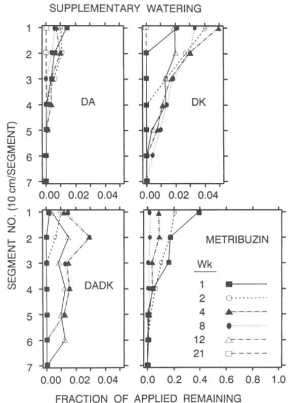
**Fig. 3.** Mobility profiles for metribuzin, DA, DK and DADK in Plainfield sand lysimeters under supplementary watering.
