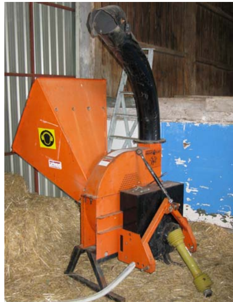
Figure 4: Wood chipper used to shred sugar beets into small enough pieces so they could be transferred into the digester.
