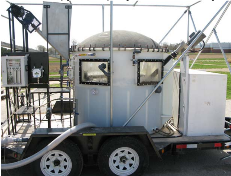
Figure 3: Digester #2 - Portable 2.2 m 3 anaerobic digester
