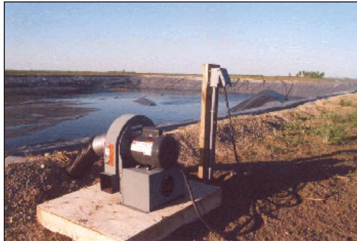
**Figure 9** This blower is connected to a ducting system so the cover remains tight on the manure surface (Hodgkinson, 2003)
