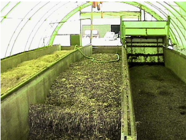
Figure 6. Overview of 3 channels - showing different carbon materials: straw, corn stalks and wood fibre.
