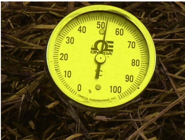
Figure 8. Thermometer showing typical temperature reached after 2 days - usual range is 55 to 70°C from day 3 to about day 14.
