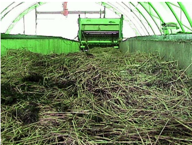
Figure 5. Turner in channel after heating has started and some settling of straw.
