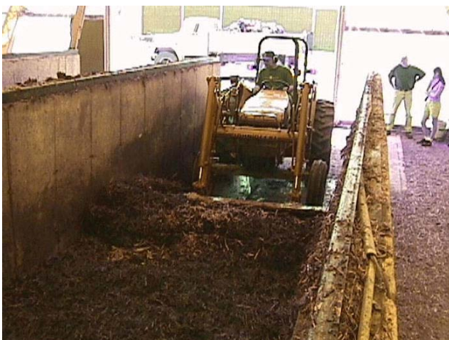
Figure 9. Removing partially finished compost from channels at about the 14-day stage - prior to the "curing" stage.
