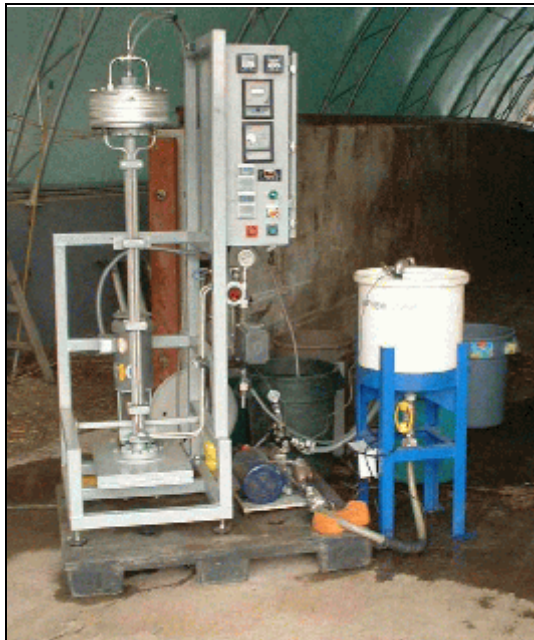
Figure 1 VSEP reverse osmosis separator
