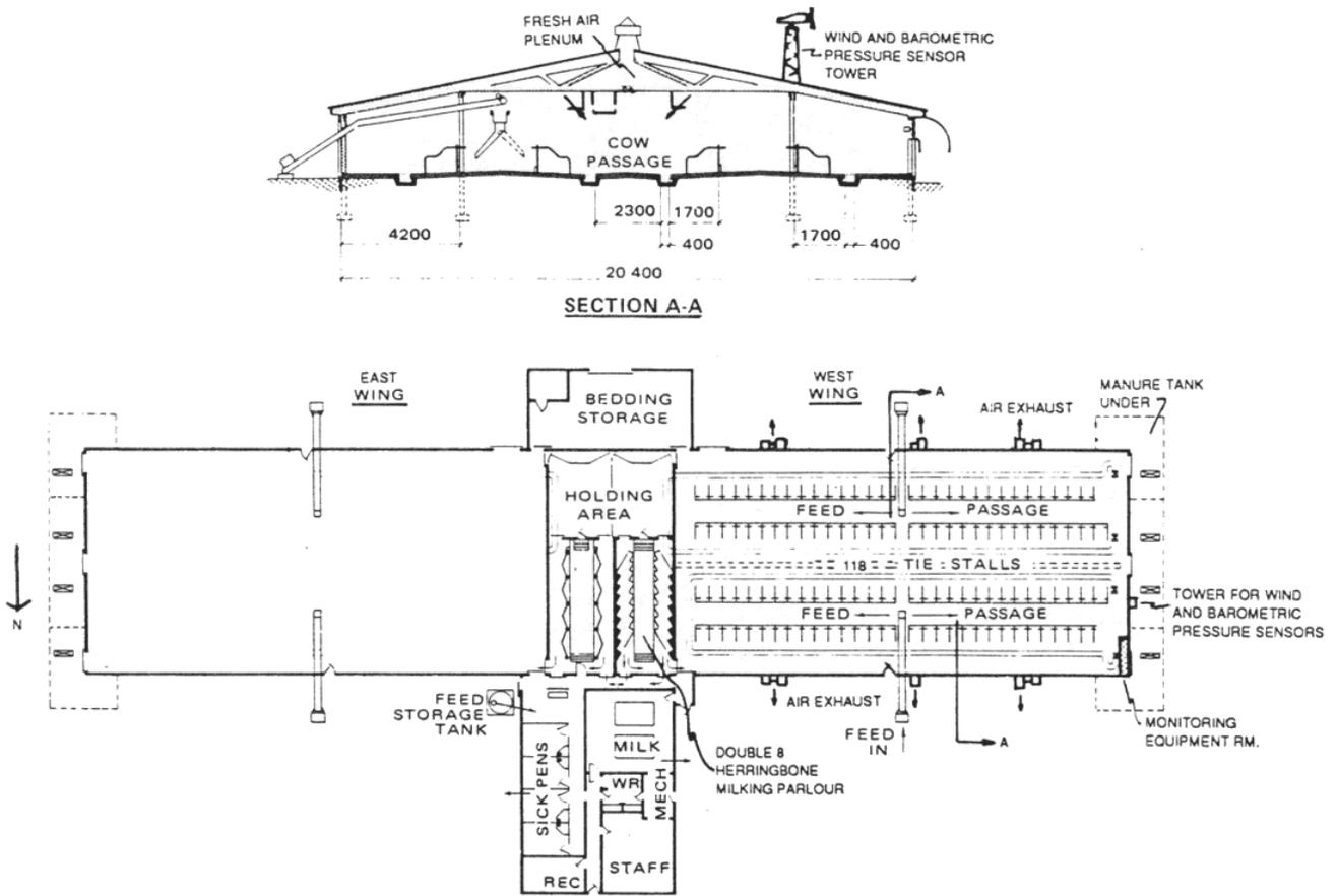
Figure 1. Floor plan and section of dairy barn used for this study
