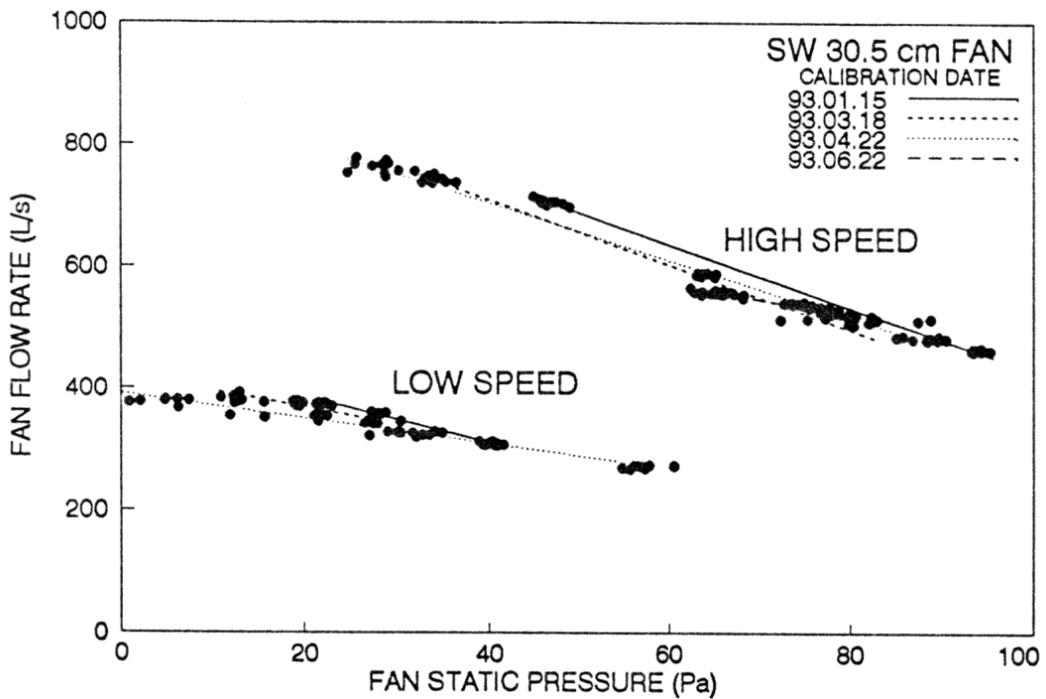
Figure 7. Fan calibration curves for the SW 30.5 cm fan
