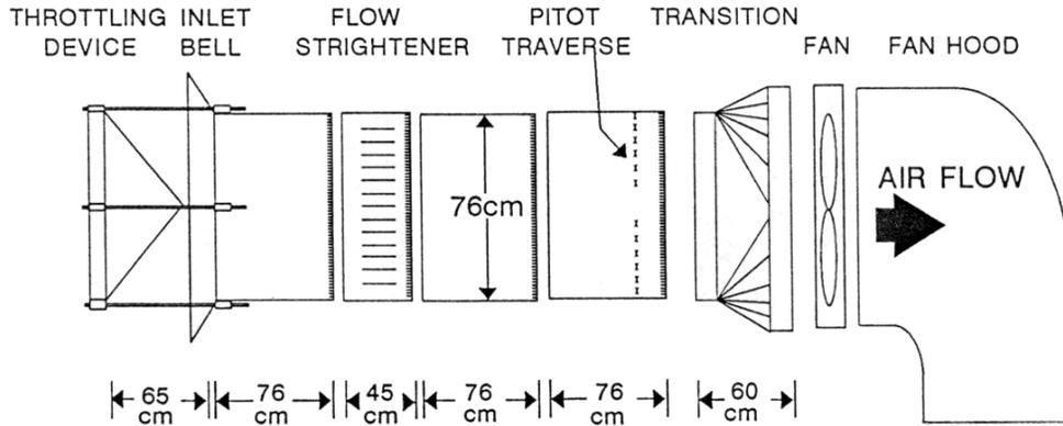
Figure 4. Fan calibration duct for the 76 cm fans
