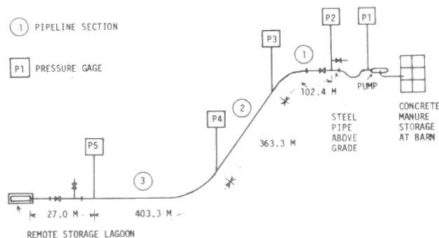
**FIG. 1 Schematic plan view of buried pipeline. Pipeline relative elevation was 6.12 m at P2, 2.73 m at P3, 1.67 m at P4, 0.46 m at P5, and 0.0 m at lagoon inlet.**
